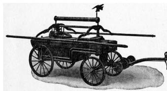
p. 354 **Engines** "The hand engines in use were the best of the kind known at the time. They had a long handle bar on each side. By working these handle bars rapidly up and down, suction and propelling power was developed. The propelling power developed in this way was strong enough to force a
